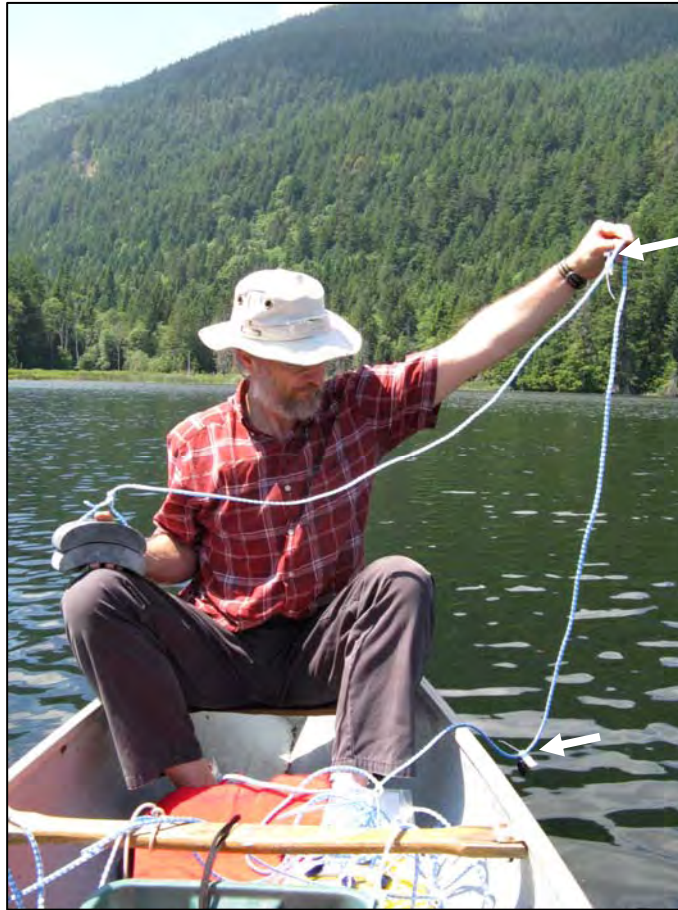
Photo 13. Deployment of recording temperature sensors in Grafton Lake. Arrows indicate individual sensors spaced at 1-m depth intervals. 18-Jul-08
