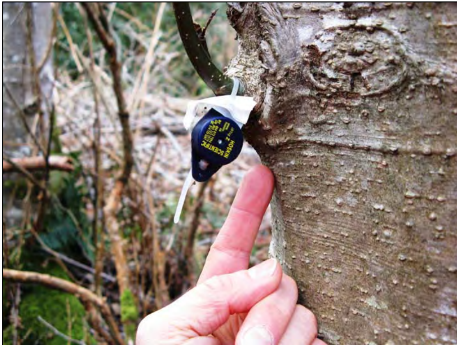
Photo 15. Close-up of temperature monitoring device (battery-powered thermister and data logger) installed to measure air temperature beside Grafton lake. 25-Mar-09
